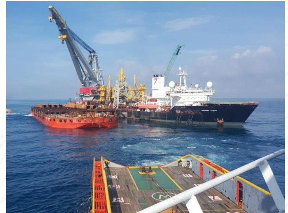
Marco Polo's MP prospect supporting the installation of monopiles of the offshore wind farm construction in Taiwan
